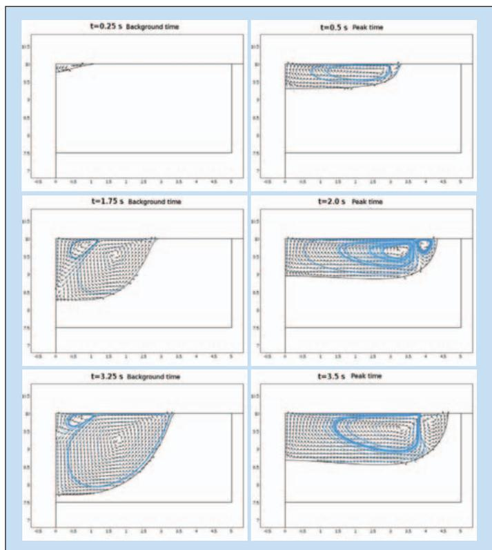
Figure 4. Time evolution of the calculated weld pool. The graph shows the case where the application of current occurs through pulses of 0.5 s each. The background currents occurs at 0.25 s, 0.75 s, etc., while the peak current occurs at 0.5 s, 1.0 s, etc....
