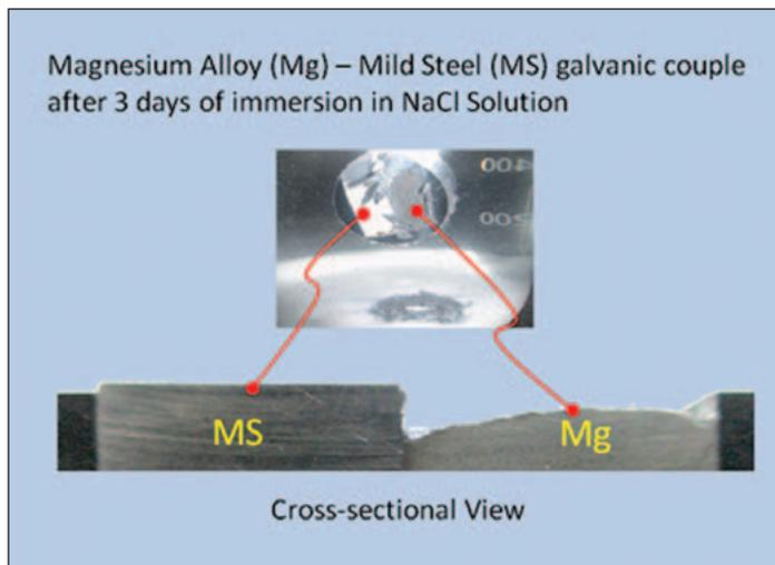
Figure 3. Corrosion of magnesium joined with steel when immersed in a salt solution.
