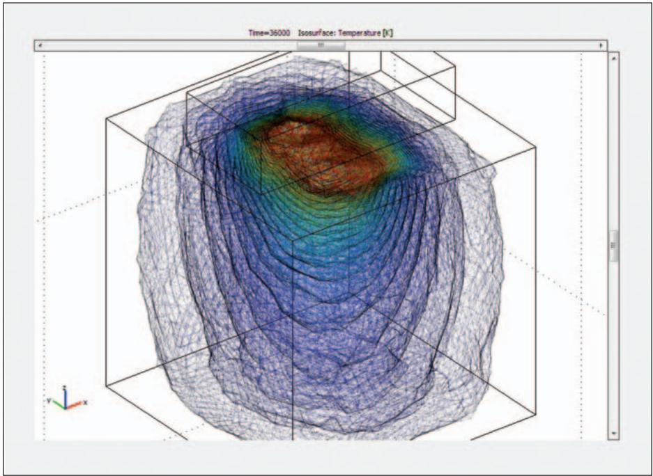
Figure 3. Transient solution of the penetration of microwave energy (0.5 GHz) into lunar soil simulant with heating of the soil. Colors represent constant temperature isotherms. The AVI movie shows the progressive heating of the soil over a period of 10 hours. Watch the movie at [http://science.nasa.gov/science-news/science-at-nasa/2009/07oct\\_microwave/](http://science.nasa.gov/science-news/science-at-nasa/2009/07oct_microwave/)
