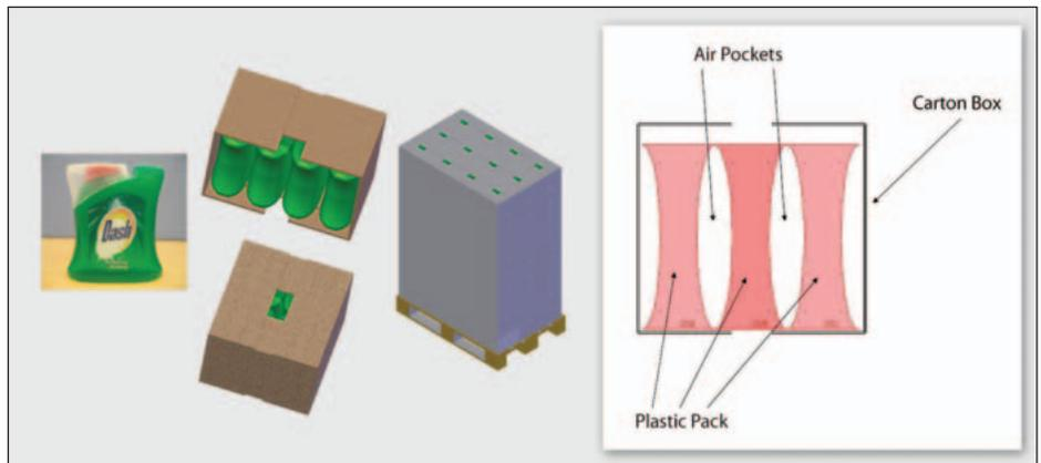
Figure 3. When consumer packages of a laundry additive are put into cartons and then packaged and placed on pallets (left), air pockets form that can potentially lead to thermal runaway.
