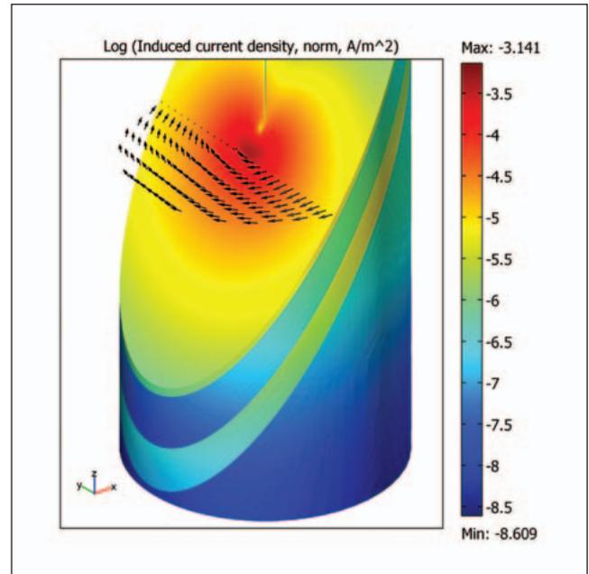
Figure 3. This image created with COMSOL Multiphysics shows a simulation result snapshot when the inductive logging tool's Z-transmitter is active at a depth of 8 feet. The subdomain colormap shows the magnitude of induced current density in the formation, while the arrows show the direction of flow of the induced currents. The colormap is log10 scaled for clarity.
