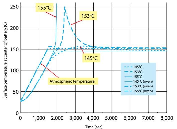
Figure 3. Change in battery surface temperature over time in heating test simulations at target temperatures: 145°C, 153°C, and 155°C.
