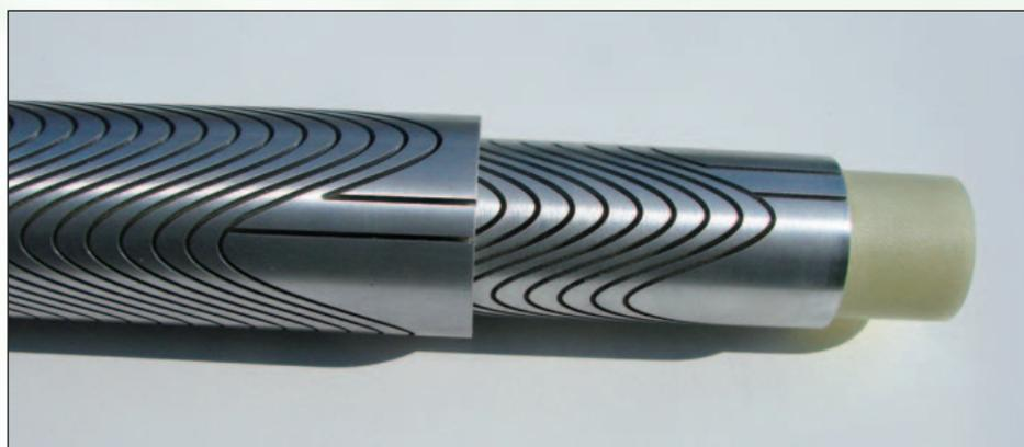
Figure 1. 2-layer multipole DDH magnet.
