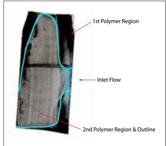
Figure 5. A cross-section from a validation sample compared to COMSOL results (blue line) shows that the outline of the second polymer matches very closely.
