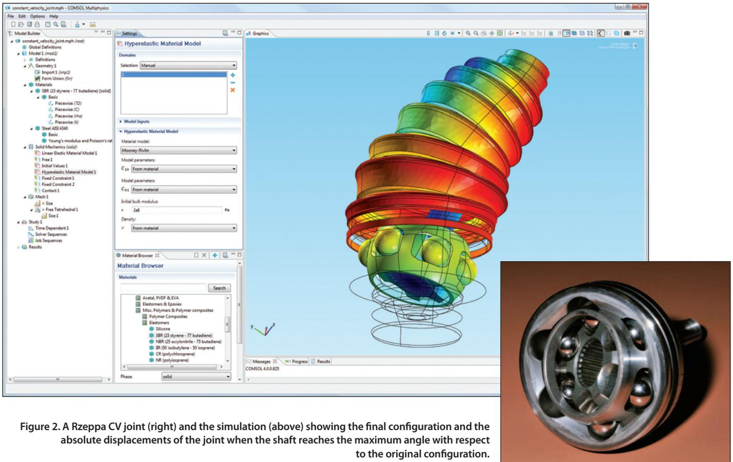
Figure 2. A Rzeppa CV joint (right) and the simulation (above) showing the final configuration and the absolute displacements of the joint when the shaft reaches the maximum angle with respect to the original configuration.
