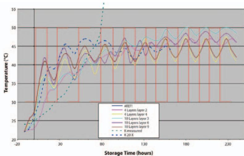
Figure 5. Comparison of actual temperature (solid lines) with model results (blue dotted line); the red pulse shows the cycling of the oven temperature.
