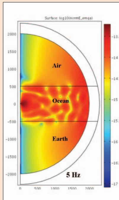
Figure 2. (left) Z component of magnetic field produced by 5Hz acoustic source 500m below ocean surface.
