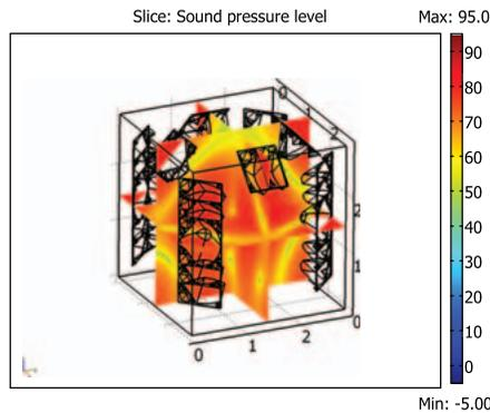
Figure 2. Acoustic signature of room containing optimized panel and material selection.
