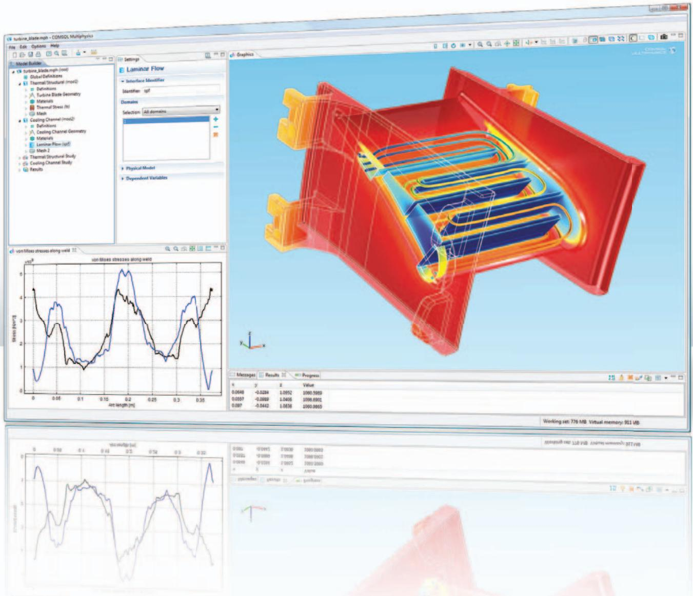
A stator blade in the turbine stage of a jet engine is heated by the combustion gases. To prevent the stator from melting, air is passed through a cooling duct in the blade. The resulting temperature gradients introduce significant stresses. Shown is the temperature distribution throughout the blade, as well as the von Mises stresses in both welds.
