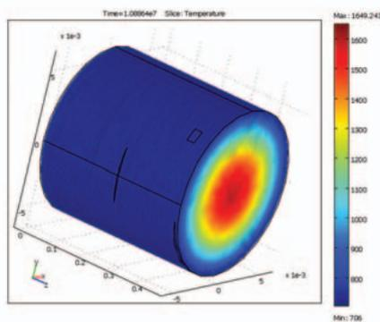
Figure 3. Temperature profile of oxidized defective fuel. Fuel element temperature slice plot in degrees Kelvin.
