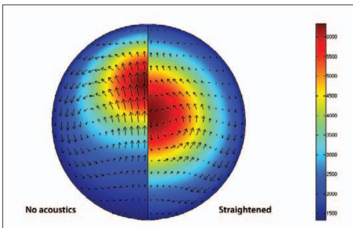
Figure 2<sup>3</sup>. Comparison of a bowed arc with an acoustically straightened arc. Temperature (K) is shown in the color map and vectors represent streaming velocity. The arc is the region of temperature greater than 5000 K.
