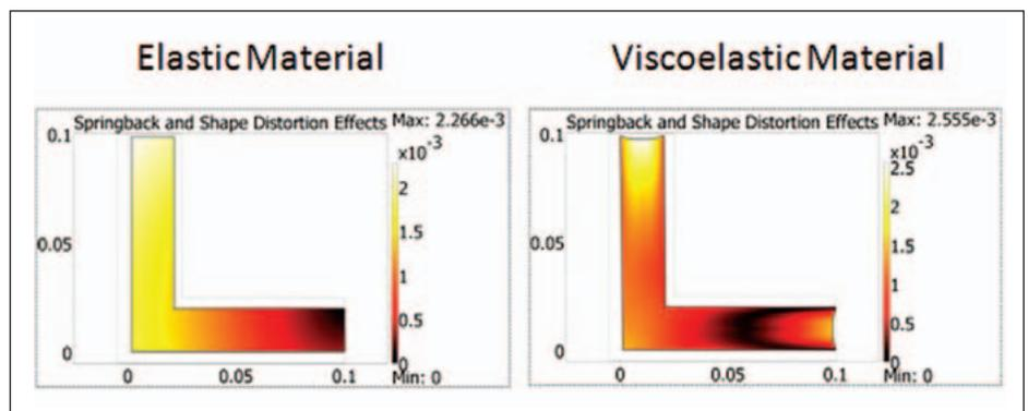
Figure 2. Viscoelastic model (right) captures the subtle influences of temperature and cure transients on the shape distortion effects.
