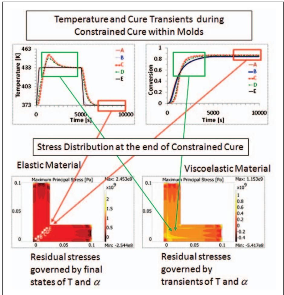
Figure 1. Residual stresses in an elastic material are only governed by the instantaneous states of temperature and degree of cure, while the stresses in a viscoelastic material are strongly governed by the thermal history experienced by the resin.
