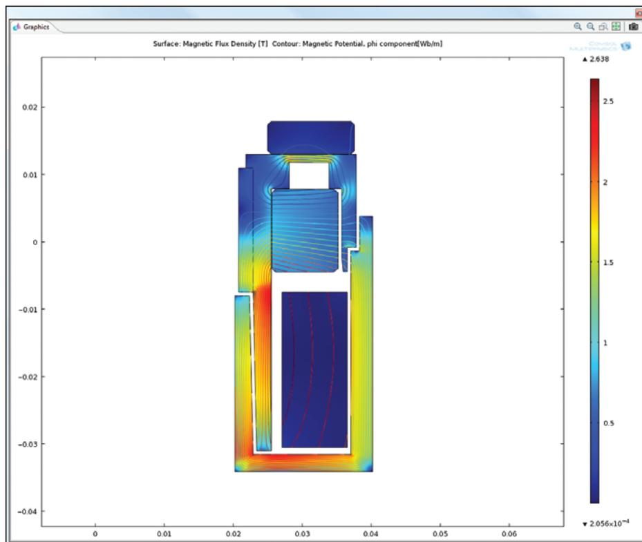
Figure 1. Surface plot of the norm of the magnetic flux density and contour plot of the magnetic potential in a clutch.
