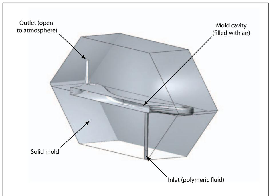
Figure 2. Modeling domain showing half the geometry for molding a dual-elastomer LARS. The polymer solution enters at the bottom and pushes air out through the top opening.
