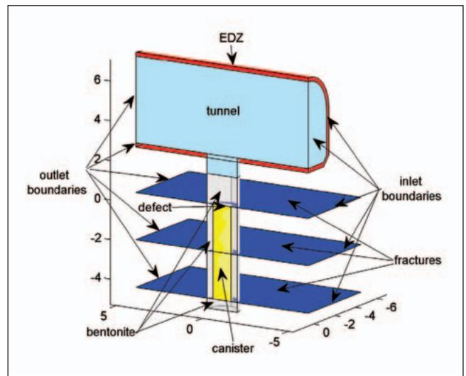
Figure 2. Modeling domains. Radionuclides seep from a defect in the canister and are transported by diffusion through the bentonite, rock fractures, the tunnel and the excavation damaged zone (EDZ).
