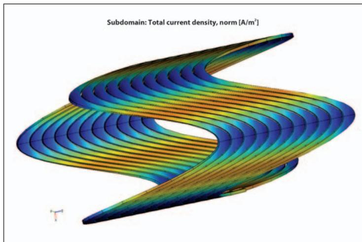
Figure 2. Current density distribution in a few turns of a 4-pole DDH magnet.
