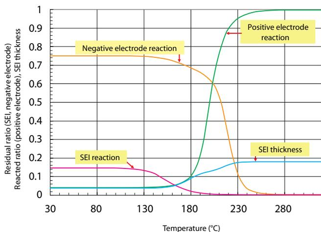
Figure 2. Analysis of reacted ratio under temperature elevation process (5°C/min) using reaction rate formula.
