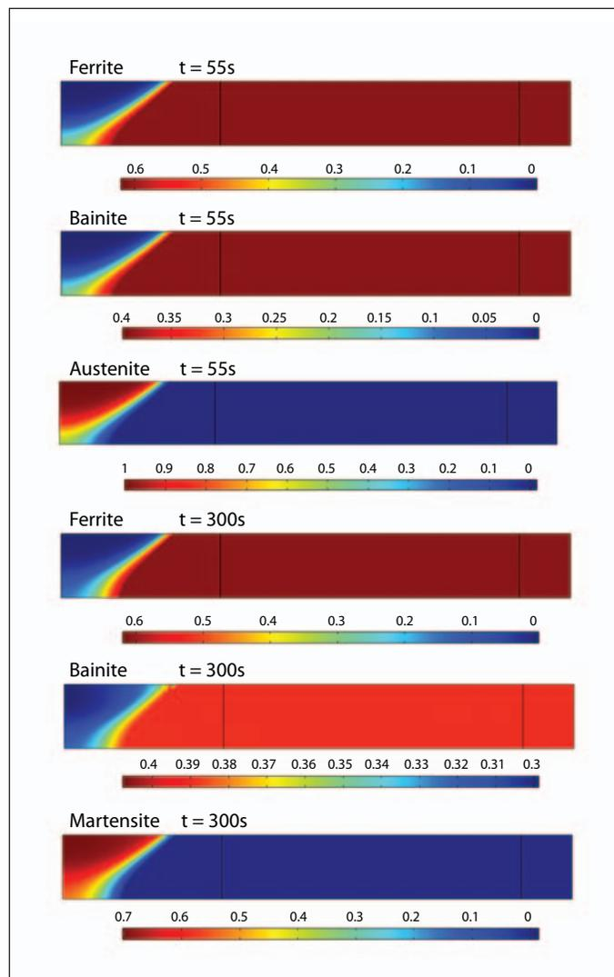
Figure 5. Phase fields in a steel disk at the end of heating ( $t = 55$  s) and after cooling ( $t = 300$  s). In the beginning, the ferritic part and bainitic part at the center were transformed directly into austenite, while after cooling a mixture of martensite and bainite is obtained.
