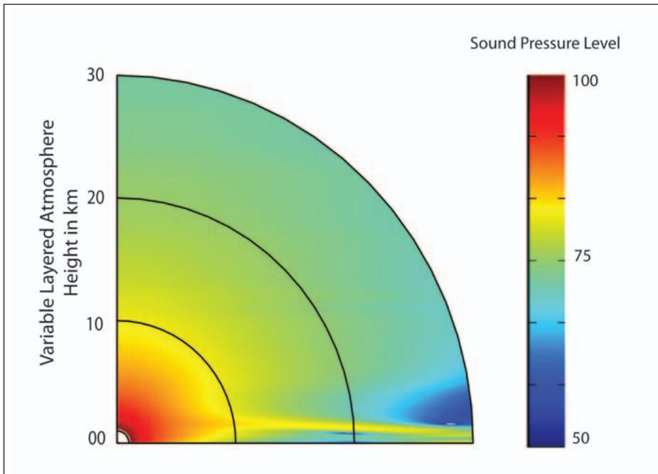
Figure 6. Energy propagation pathways through the lower atmosphere for regional propagation at 2 Hz.
