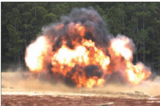
Figure 5. Above ground detonation of 100 lbs of ANFO from calibration experimentation.
