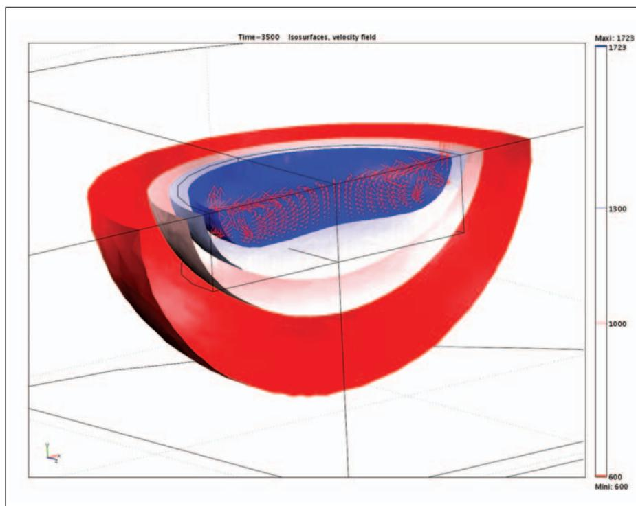
Figure 2. 3D representation of the weld pool at the end of the heating duration and some iso-thermal lines.
