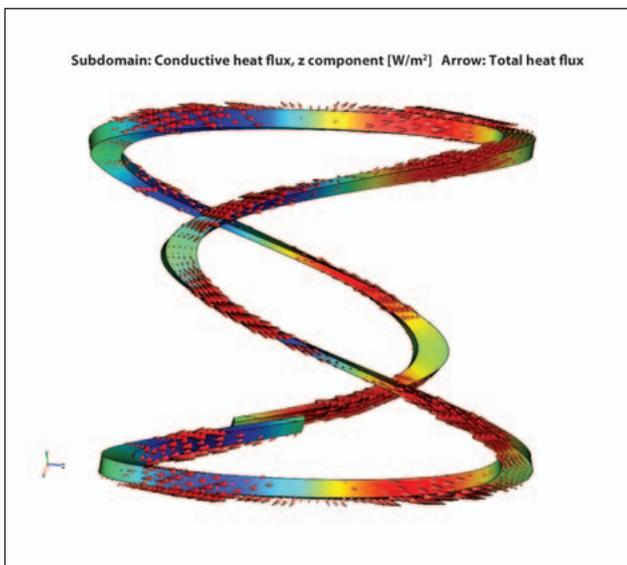
Figure 3. Heat flux distribution in one turn of a 4-pole DDH magnet.
