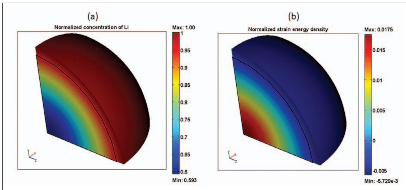
Figure 4. Typical 3D results from COMSOL Multiphysics simulations of a nodular battery electrode particle, idealized as a sphere. It shows the subdomain contours of (a) the normalized lithium concentration and (b) normalized strain energy density during intercalation of lithium into the host material while the battery is being charged or discharged. The black outline is indicative of the initial shape and size of the particle. Deformation is scaled for clarity.
