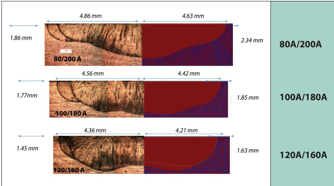
Figure 3. Comparison between the experimental macrographs of the three pulsed current cases (left) and the predicted weld pool shape after solidification (right), which shows very good agreement in both shape and dimensions.
