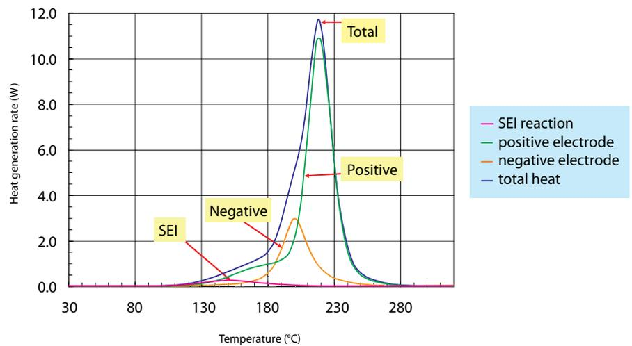
Figure 1. DSC measurements of heat reaction of active Materials
