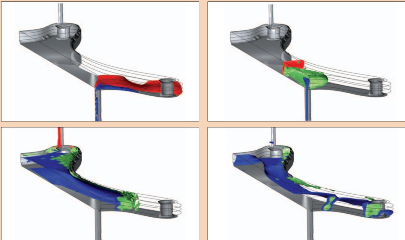
Figure 3. Simulation of the polymer as it fills the mold cavity after 20s, 40s, 100s and 3000s. The red isosurface indicates where the boundary between the polymer mixture and air occurs, the green isosurface indicates where the volume fraction between the two polymers is at 50%, while the blue isosurface is where the second polymer has a volume fraction of 100%. Note that some of the mold cavity walls have been removed for illustrative purposes.
