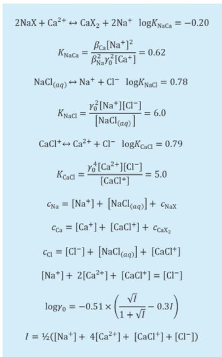
Figure 4. Chemical reactions and equations involved in describing the transfer of sodium and calcium ions between the bentonite and water.
