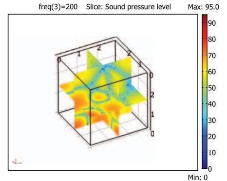
Figure 3. Acoustic signature of room not optimized for acoustic response.
