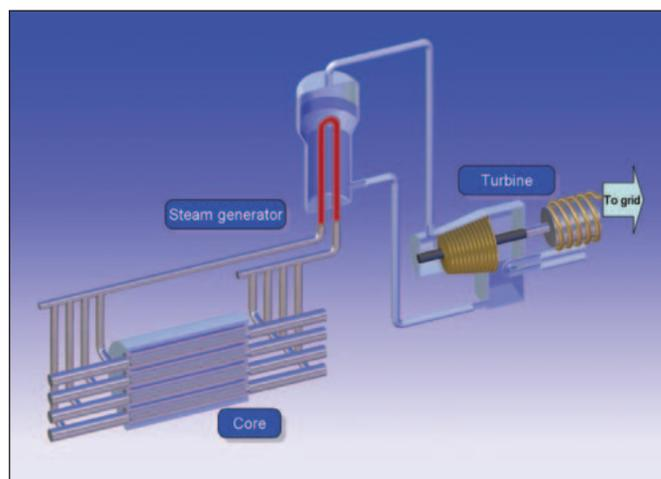
Figure 1. Schematic of a CANDU plant. Used with permission from A. El-Jaby.
