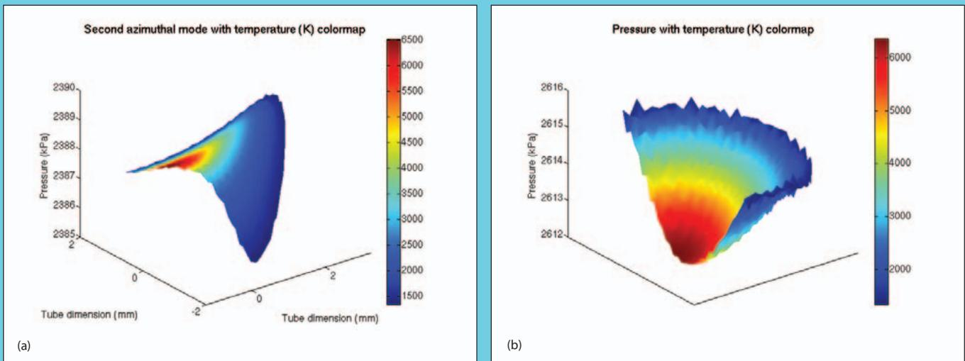
Figure 4<sup>3</sup>. Pressure modes that are needed for arc straightening. The second azimuthal mode (a) initially causes streaming flows that lower the arc from its bowed position. The first radial mode (b) causes streaming flow that holds the arc close to the center.
