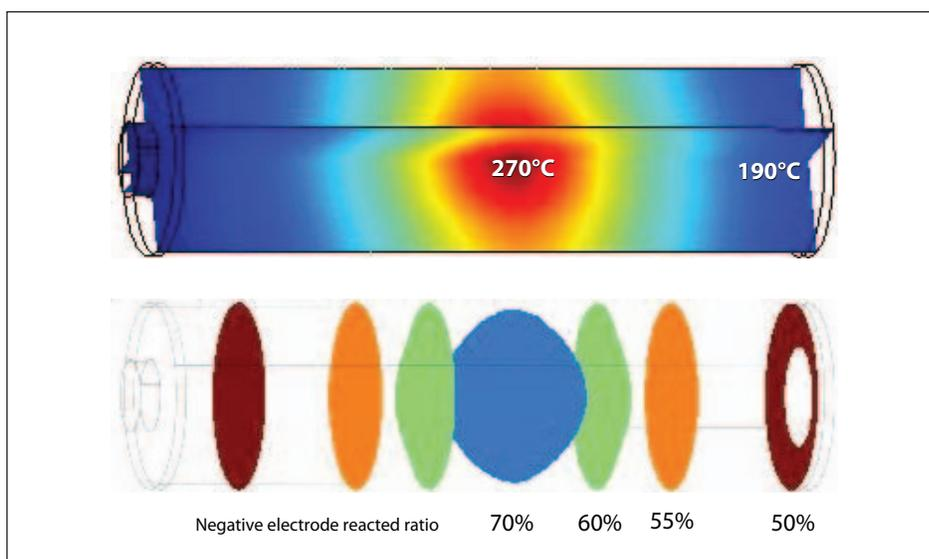
Figure 4. Internal temperature at start of thermal runaway for target temperature of 155°C (190–270°C) (above) and isosurface of negative electrode reacted ratio (below).
