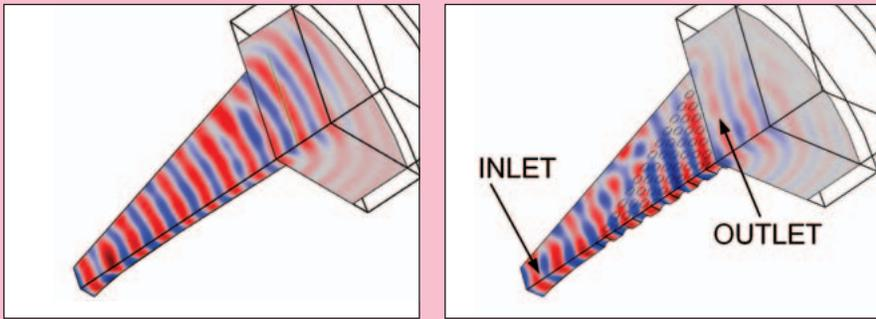
Figure 2. These images, created with the Acoustics Module for COMSOL, show the sound pressure level at 16 kHz through the waveguide. Here the two cases solved for are: no acoustic lens embedded (left), and the final prototype with the lens showing how the wavefront is almost perfectly planar at the waveguide outlet.
