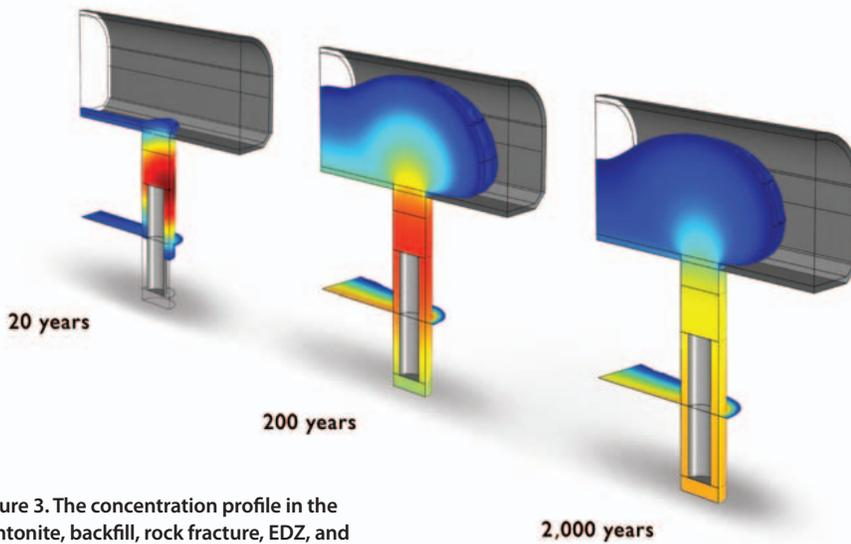
Figure 3. The concentration profile in the bentonite, backfill, rock fracture, EDZ, and tunnel after 20, 200 and 2,000 years.
