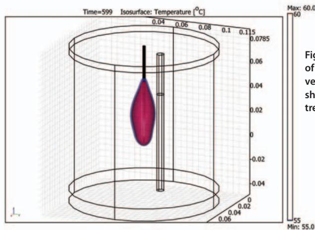
Figure 2. 3D COMSOL model of the impact of a large blood vessel on the ablation size and shape for a microwave tumor treatment.
