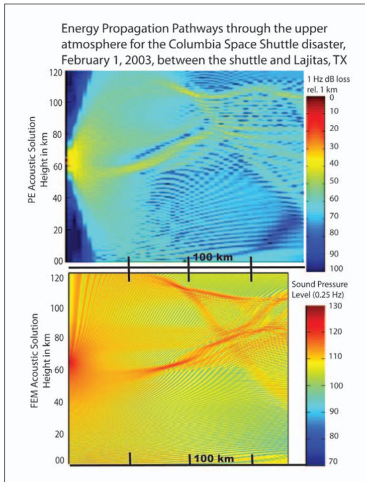
Figure 3. The PE solution for the Columbia, above. 1 Hz was taken to be the dominant frequency for modeling, determined from the observed data. COMSOL FEM Acoustics Module solution, below, for the effective sound speed profile seen in figure 2, 0.25 Hz dominant frequency.
