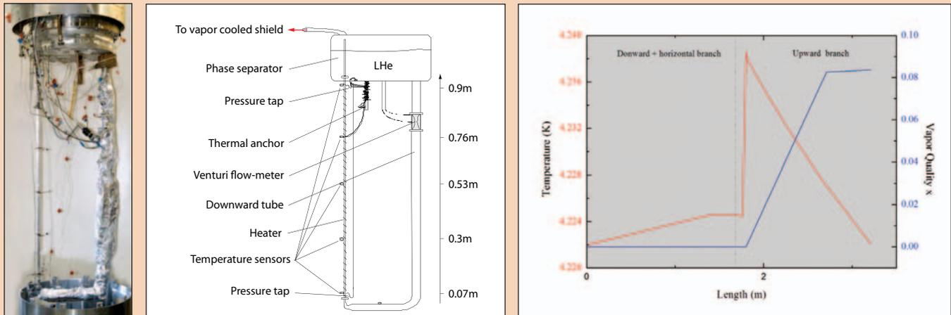
Figure 2. A photo of the small scale cooling loop (left) and a diagram illustrating its components (center). On the right are results from the 1D model show the temperature and vapour quality throughout the loop: 1- liquid helium tank; 2-downward and bottom pipe; 3-upward pipe.
