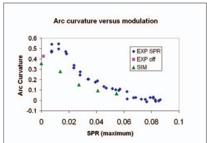
Figure 3<sup>3</sup>. Arc curvature versus spectral power ratio (SPR), a measure of the amplitude of acoustic excitation. Curvature is normalized by the arc-tube inner radius.
