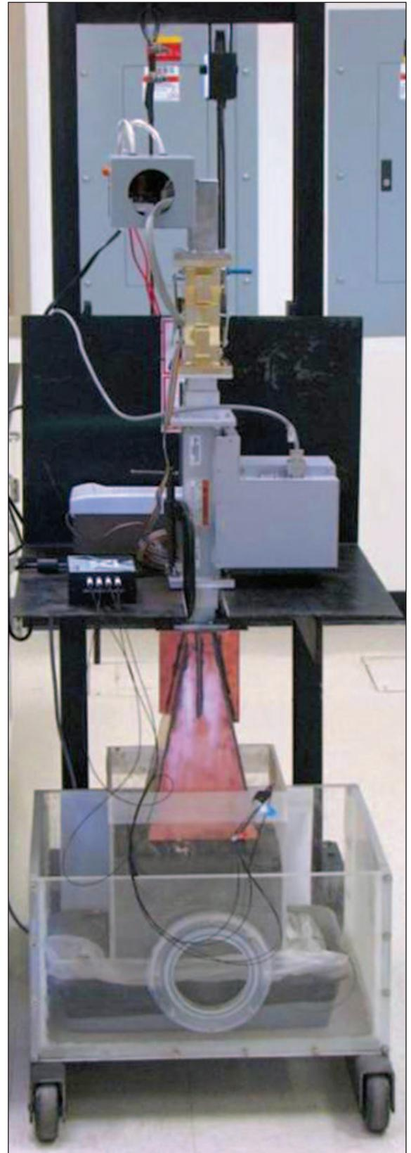
Figure 2. Demonstration hardware to test the beaming of microwave energy down into lunar soil simulant (in the box) with the microwave hardware mounted on a mobile platform. Initial test of the coupling of microwave energy into the simulant.
