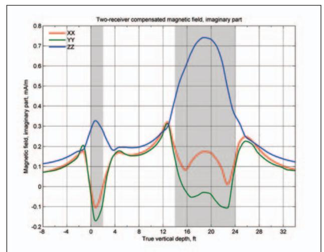
Figure 2. Imaginary magnetic fields, all three direct components, for frequency 20 kHz and when the tool is centered in the borehole. The lower frequency corresponds to a larger region of investigation. The gray shaded regions indicate the oil-bearing layers.
