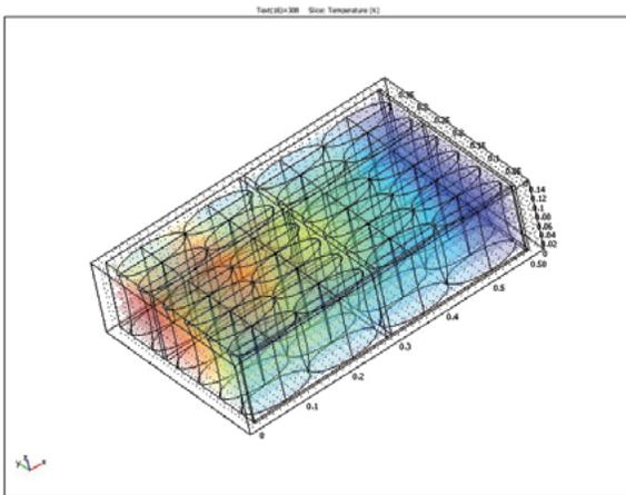
Figure 4. Temperature profile of palletized products.
