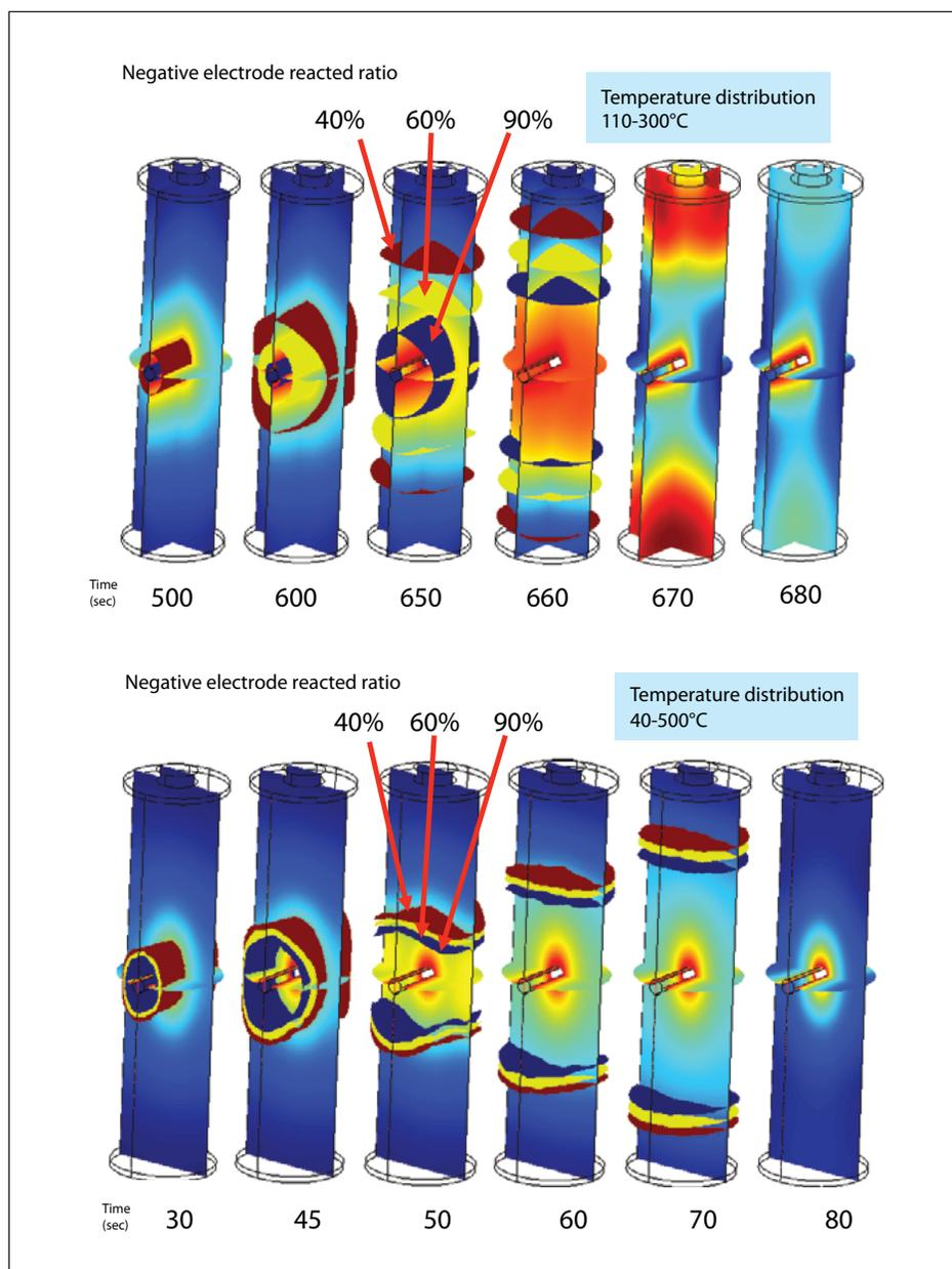
Figure 5. Change over time of temperature distribution (color contours) and isosurfaces of reacted ratio of the negative electrode during thermal runaway for an internal short circuit heat generation of 20W (upper row) and 100W (lower row).
