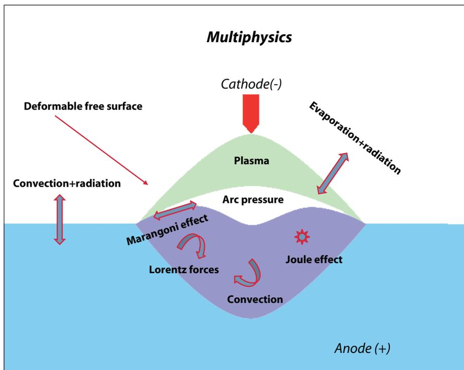
Figure 1. The primary physical phenomena in arc welding. Fluid flow in the pool is driven and influenced by a combination of buoyancy, electromagnetic forces, surface tension and arc pressure.
