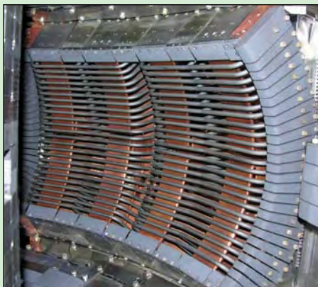
Ion Cyclotron antenna as seen from inside of the Alcator C-Mod vessel. Four copper straps stand behind Faraday shield rods which have the purpose of screening the electric field components which are parallel to the magnetic field lines.
