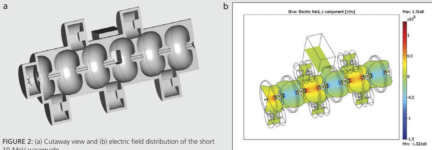
FIGURE 2: (a) Cutaway view and (b) electric field distribution of the short 10-MeV waveguide.
