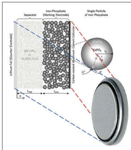
FIGURE 3: Modeling of the half cell at macroscopic (left) and microscopic (right) level.
