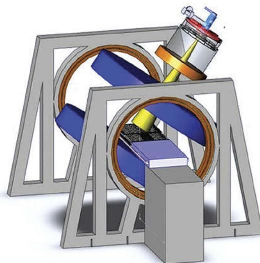
FIGURE 1: Configuration of the Linac MR system.
