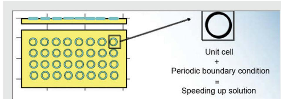
FIGURE 2: PBC functionality from COMSOL significantly speeds up the solution to our FSS study by simulating only a unit cell.
