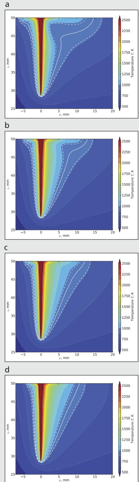
FIGURE 1: A plot of temperature in the symmetry section of a weld shows that without any magnetic field applied (a), the weld takes on a wine glass shape. With the addition of a magnetic field ( $b = 0.50$  T,  $c = 1$  T and  $d = 2$  T), the shape starts to take on the form of a V.
