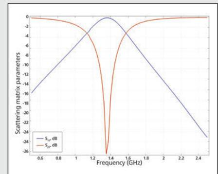
FIGURE 6: Reflection and transmission parameters of the fractal spiral resonator.
