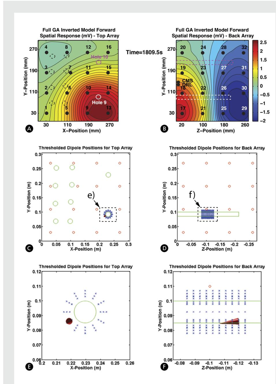
FIGURE 3: Forward-modeled voltage distribution of a dipole for one event (a and b), Spatial location of the dipole within the concrete block (c and d), Close-up of the dipole location (e and f), showing an off-vertical orientation of the dipole moment.
