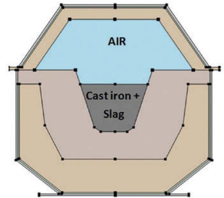
FIGURE 2: 2D geometry of a roof runner. The molten metal comes in contact with a concrete liner, and the outer shell is of cast iron.
